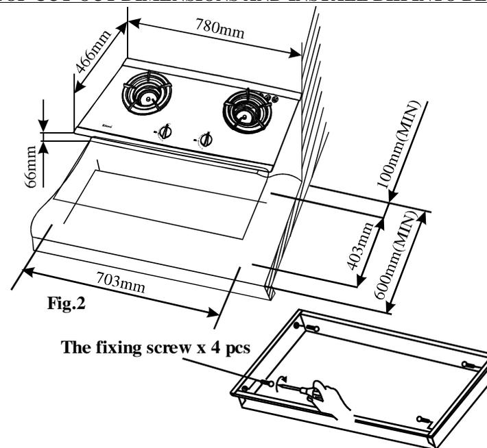
Confirm fourscrews are securely into the casing.
